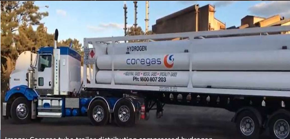
Image: Coregas tube trailer distributing compressed hydrogen
