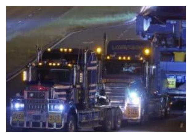
Heavy haulage specialist Lampson Australia was involved with the move, which was coordinated together with Transport for NSW. It provided the two Kenworth T509s to do the pulling. While a Mack Titan and Kenworth C501 were at the back, doing the pushing. Overall, the monster combination measured 121 metres long, 5 metres wide and 5.7 metres high – with a total mass of 786 tonnes.
