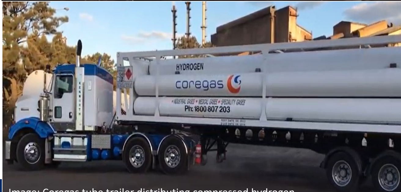
Image: Coregas tube trailer distributing compressed hydrogen
