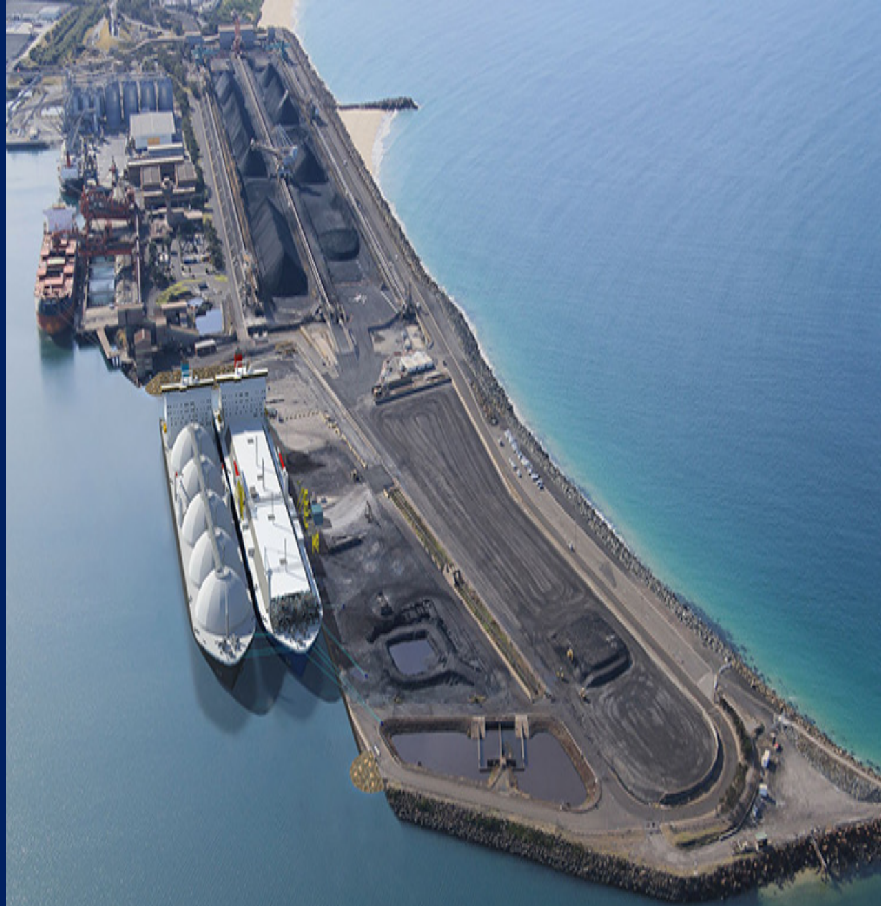
Image courtesy of Squadron Energy - Port Kembla Energy Terminal site with permanently moored FSRU with LNG carrier alongside to deliver its cargo
