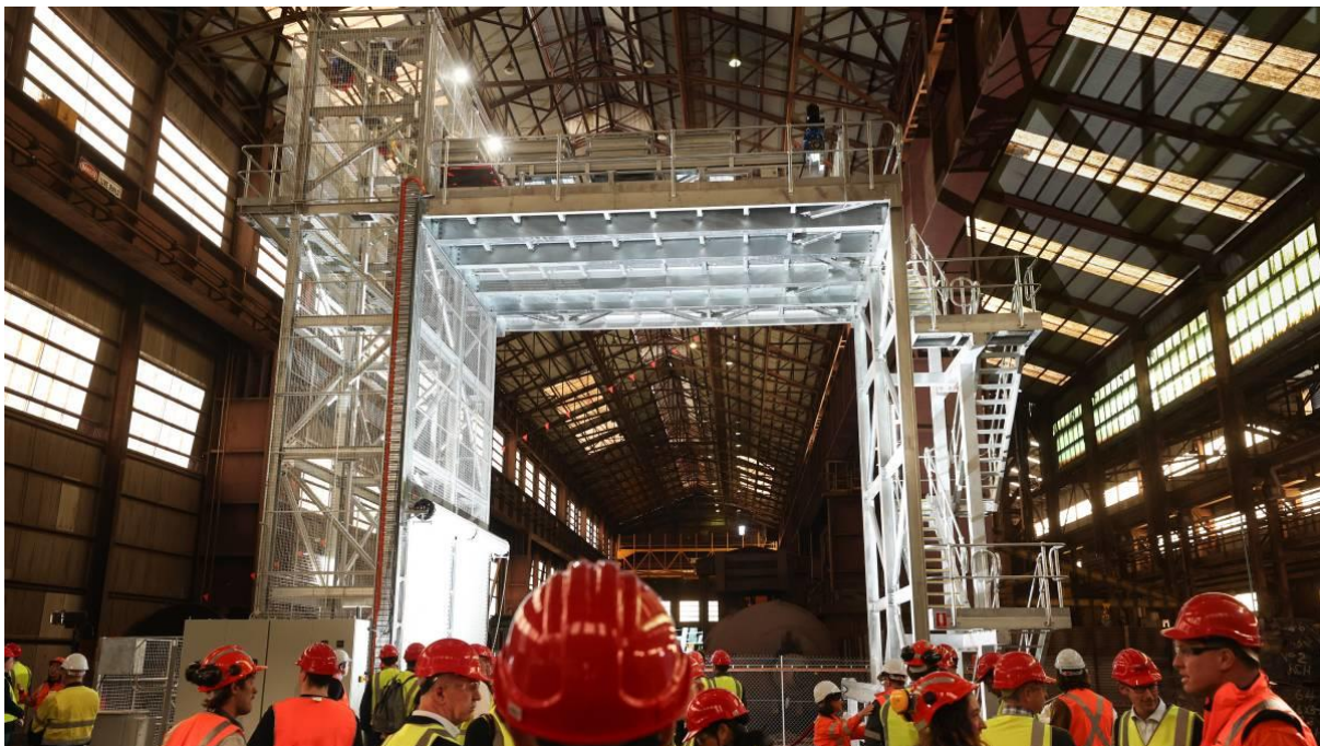
Green Gravity's GravityLab - a 1:30 model of the proposed energy storage system. Picture by Adam McLean
