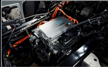
Hydrogen Fuel Cell System
